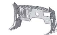
Single-part casting concept: In high-pressure die-casting
